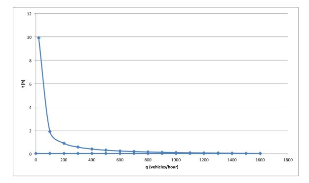
t is not a single-valued function of q (as we have seen from the relationship between them and the figures above) because the same flow rate q can be achieved at two different times t and densities k.
