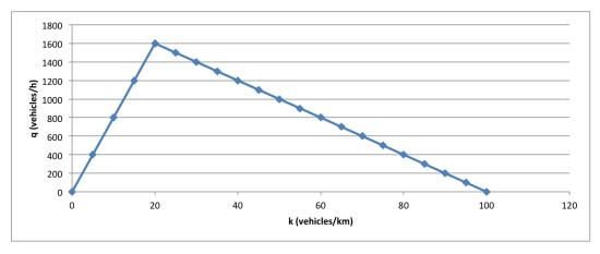
(b) Consider a 2-kilometer stretch of this highway. Plot the t vs. q relationship for a car traveling on one of the lanes of this highway for all the possible values of q. In other words, show on the vertical axis the amount of time it will take to travel this 2-kilometer segment for all possible values of q. Is t a single-valued function of q?
